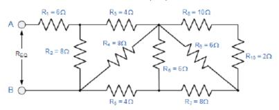
Determine resistance between the points A & B. Determine the power supplied by voltage source if 25V is connected across A & B.
